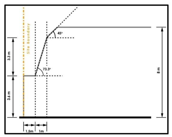
Figure 2: Diagram of GRZ-R5. 2 Alternative Height in Relation to Boundary Rule
